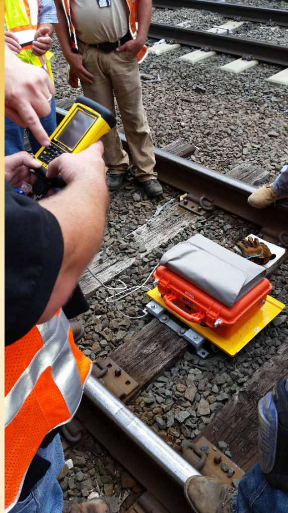
Transponder testing with Portable Testing Equipment (PTE)
